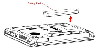
Figure 6-2 Removing the battery pack
